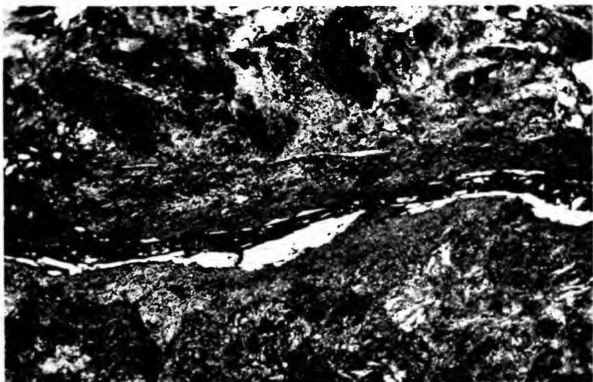
Fig. 4 (Investigation 132-108)—Photomicrograph of a specimen cut longitudinal to the rail in a vertical plane through the nucleus (origin being a shell) of the detail fracture shown in Fig. 3. The presence of an unidentifiable foreign material outlining this shelly crack can be noted at a magnification of 250X. Etchant, 3 percent nital.
